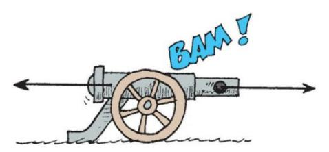
The force exerted against the recoiling cannon is just as great as the force that drives the cannonball inside the barrel(Newton's 3rd Law).
