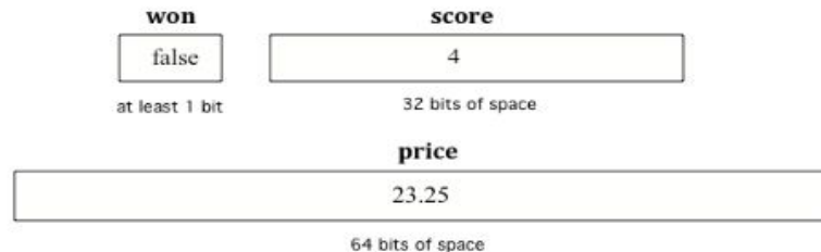
Figure 1: Examples of variables with names and values. Notice that the different types get a different amount of space.
