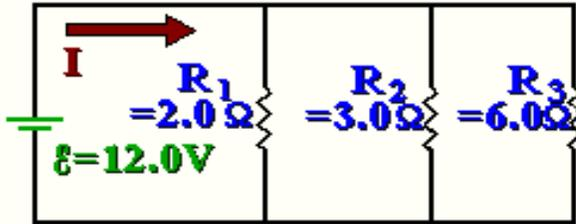
**Figure 1** Example Problem: Resistors in Parallel
