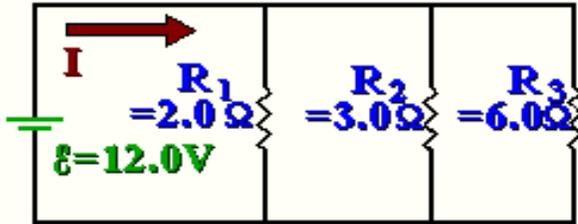
**Figure 1** Example Problem: Resistors in Parallel
