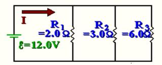
Figure 1 Example Problem: Resistors in Parallel
