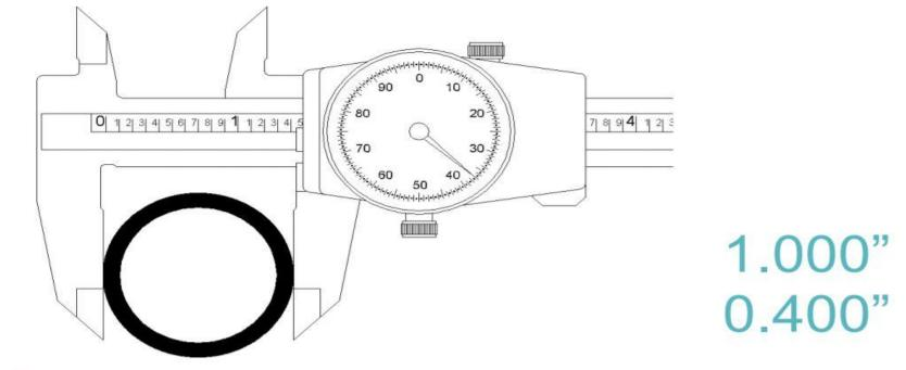
The *reference edge* is located between the 1 and 2 inch marks. So, the user makes a mental note...1 inch.
