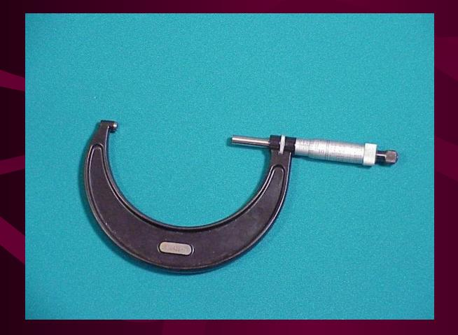
• Read the largest numbered line showing on the barrel.
