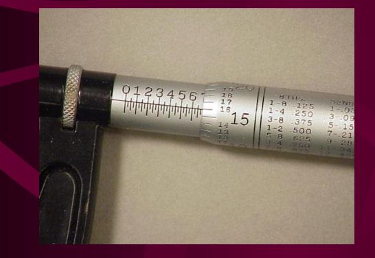
• Read the largest numbered line showing on the barrel.
