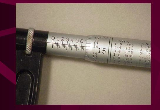
• Count the small lines between the long 6 line, and the edge of the thimble.
