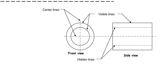
3. <u>Center Line</u>: center lines are a thin line with one short dash between two long dashes. They are used to show the centers of holes, arcs, and symmetrical parts (symmetrical means both sides are identical). Sometimes you will see the symbol CL, to designate a centerline, and SYM to tell you the part is symmetrical around the centerline.
