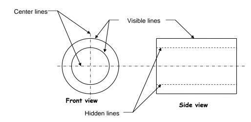
3. <u>Center Line</u>: center lines are a thin line with one short dash between two long dashes. They are used to show the centers of holes, arcs, and symmetrical parts (symmetrical means both sides are identical). Sometimes you will see the symbol CL, to designate a centerline, and SYM to tell you the part is symmetrical around the centerline.
