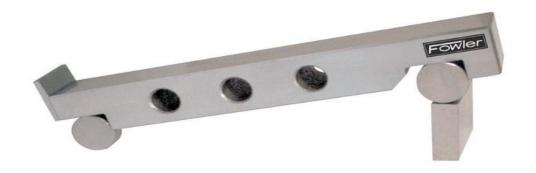
Two cylinders of equal diameter are placed at the ends of the bar. The axes of these two cylinders are mutually parallel to each other, and are also parallel to, and at equal distance from, the upper surface of the sine bar. Accuracy up to 0.01mm/m of length of the sine bar can be obtained.
