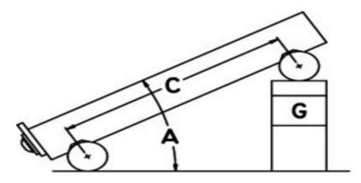
If you just want to set an angle with a sine bar and stack of blocks, then take the sine of the desired angle on your calculator and multiply the result by the distance between the centers of the cylinders in the sine bar. Assemble a stack of blocks equal to this value and put it under one of the cylinders.
