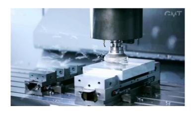
Face Milling is used to create flat surfaces and contours on the finished piece and is capable of producing higher quality finishes than other milling processes.
